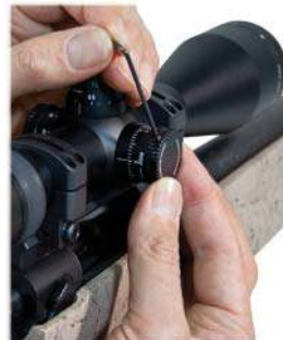
Align the windage turret cap.
