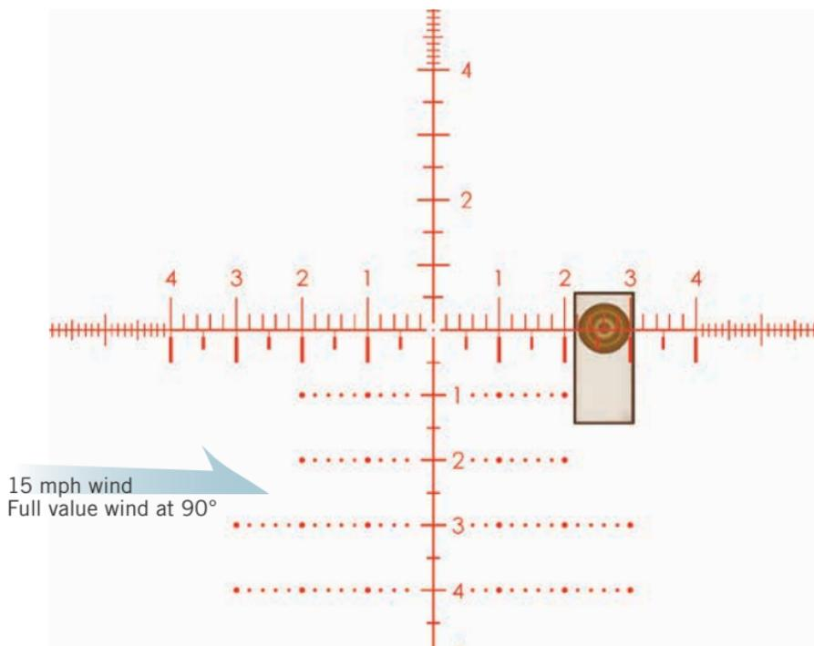
2.6 MRAD correction for 15 mph wind at 700 yards. Elevation already dialed into turret.
