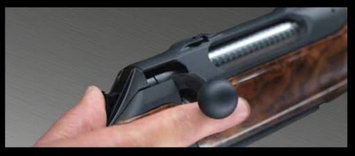
Good enough isn't enough: In addition to the manual cocking feature, an automatic firing pin safety works inside the S404 to prevent it from firing when the bolt is not fully closed. In order to open the bolt with the gun on safe – e.g. to load and unload – it is only necessary to push the cocking slide forward two millimeters while at the same time lifting the bolt handle. This way, safe handling becomes instinct aided by intelligent technology.
