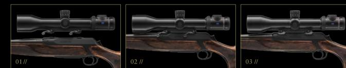
Good things come in threes: The SUM mounts effortlessly onto the S404. 01// Tip the scope to the side so that the crossbars of the mount engage the milled slots in the receiver. 02 // Push the scope toward the muzzle and lock the rear lever. 03 // Lock the front lever.
