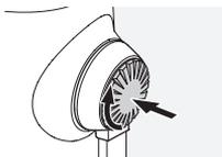
Push the knob in firmly and rotate slightly clockwise.
