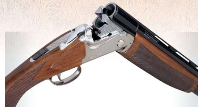
The Instinct SL receiver is fitted with automatic ejectors and features a locking bolt that emerges from the bottom of the standing breech to engage a recess machined into the barrel monobloc.
